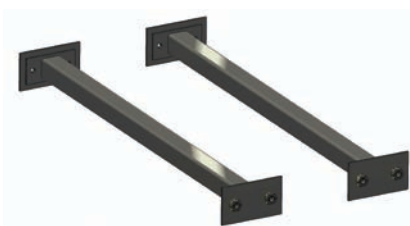
F14 Universal seat subframe to be adapted to the vehicle body floor according to FIA 253-65B Annex J instructions. - 2x 35 mm squared section pipes - 4x end plates (90x45) mm - 4x steel plates (110x65) mm - 4x M8 bushing RFST0079
